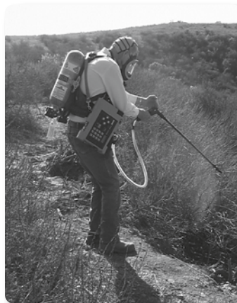
Mundt uses toxic vapor analyzer equipment to check on a reported leak in a gas line in an oil field.
