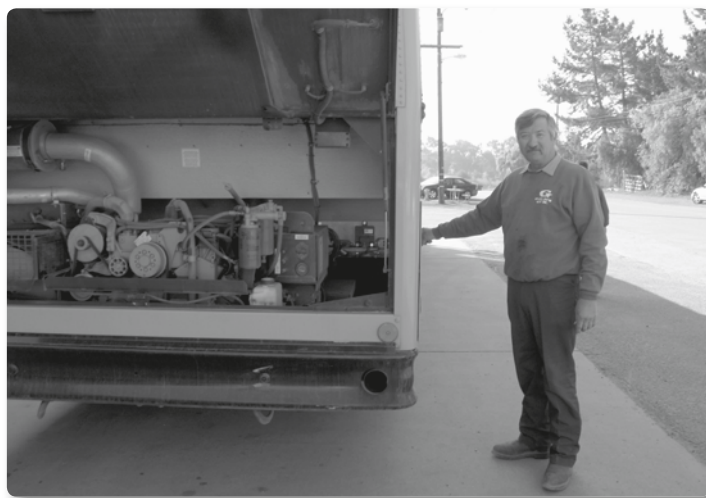
Orcutt School District Head Mechanic Garwin Weiting, with one of the school buses recently outfitted with a particulate trap, which will cut 85 percent of the diesel particulate emissions from the exhaust. Weiting is demonstrating a side panel where the driver can see if it's time to clean the trap. If so, it is replaced with a clean one kept on hand, and the dirty one is sent to a facility in Los Angeles, which cleans it and returns it.
