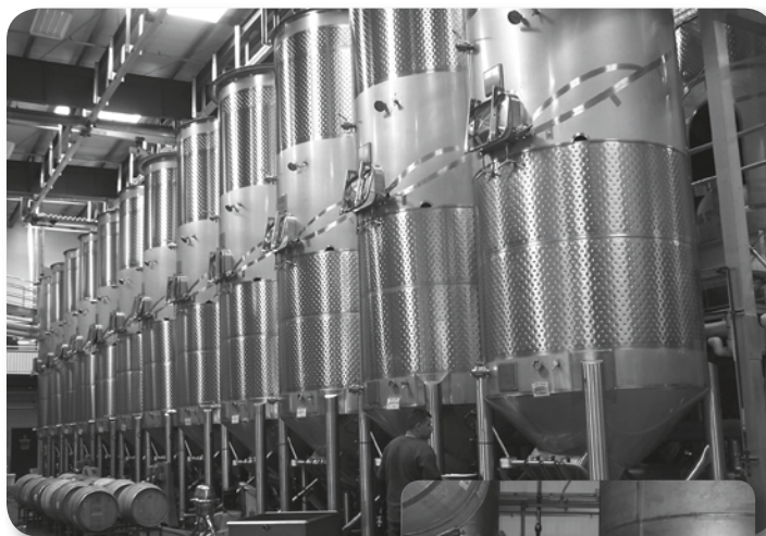
Tanks at the facility hold up to twenty tons of wine (for the red wines).
