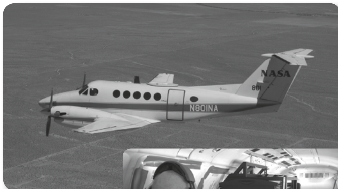
The thermal-infrared wildfire scanner is mounted in a NASA Beechcraft B200 King Air twin-turboprop plane. Photos courtesy of NASA, Lori Losey, and Mark Pestana.
