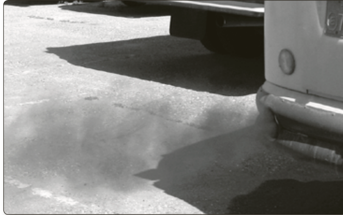
One of the older school buses that is being replaced releases a plume of soot when its engine is started (above). It also has to idle for several minutes before its engine shuts off. The new buses don't emit plumes of soot, and don't need to idle before shutoff.
