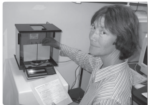
APCD Monitoring Specialist Janice Kettler weighs filters in APCD's monitoring lab to arrive at a determination of the levels of particles less than 10 microns in diameter (PM10). Levels of PM10 are monitored at six stations throughout the county, while levels of particulate matter less than 2.5 microns in diameter (PM2.5) are monitored at stations in Santa Maria and Santa Barbara
