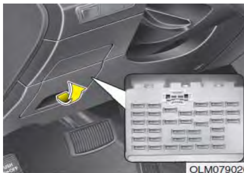
Conventional vehicle system related fuses and relays
