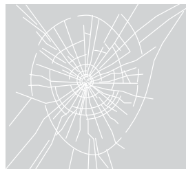
< Broken Laminated Glass >
