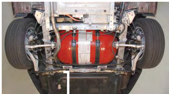
Hydrogen Pressure Relief Tube Location
