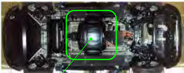
Battery system → underneath the vehicle(center)
