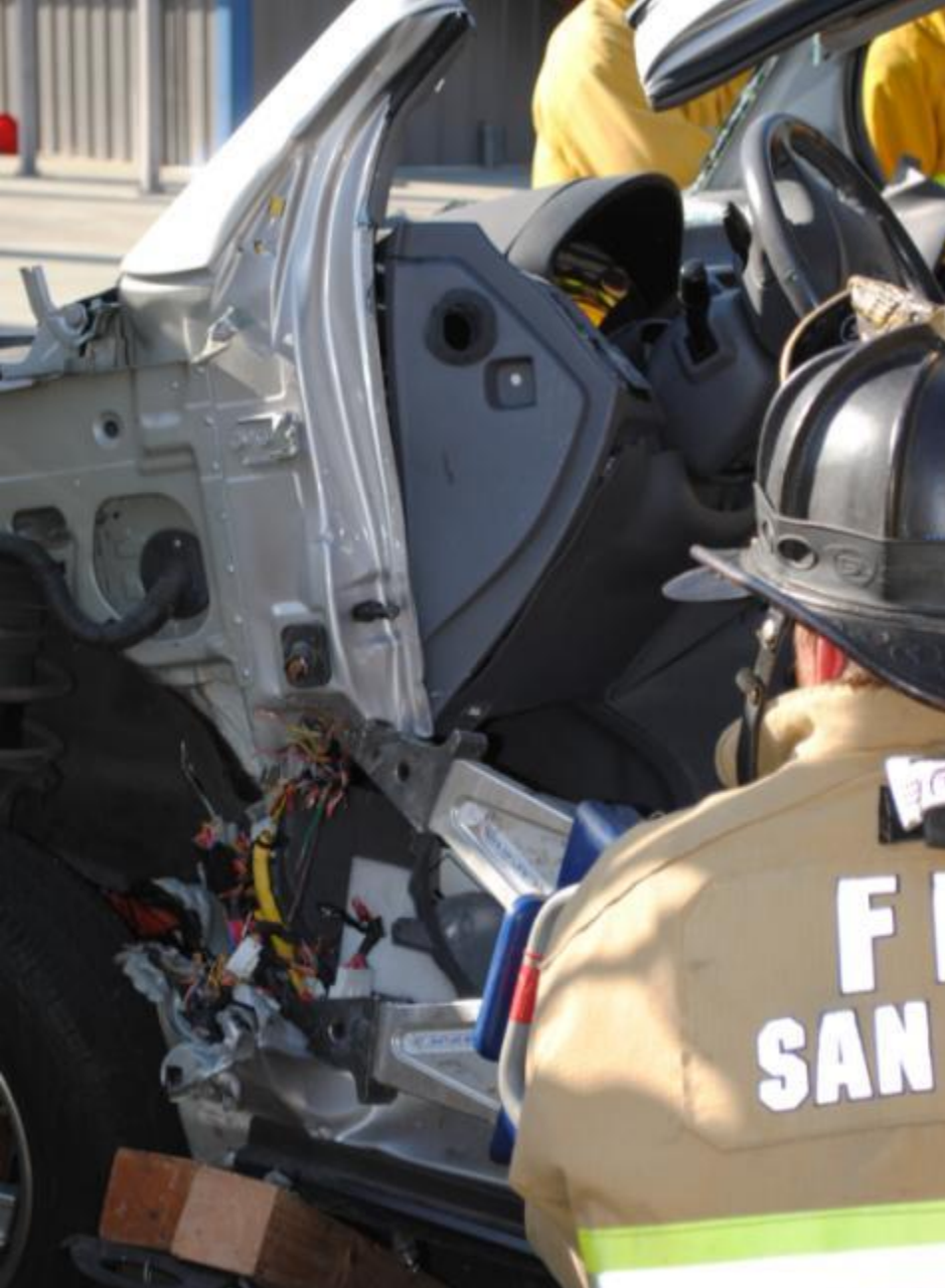
Showing a dash roll by cutting A-pillar and pushing with spreaders (no high voltage cables present)
