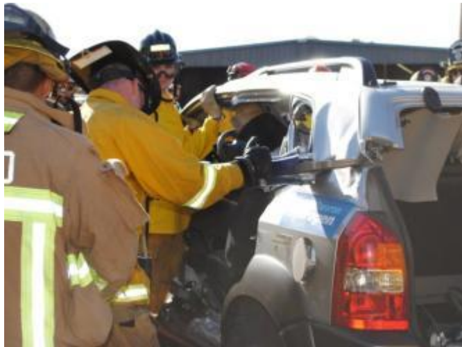
Removing the roof; no H 2 vent lines in the C or D pillars/posts, already did the "peel & peek" for airbag cylinders
