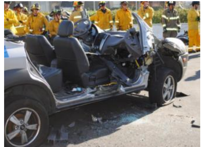
After the demo: all doors, hood, and roof removed, and dash rolled
