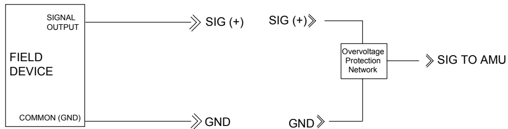
TYPICAL 2 WIRE 4--20mA FIELD DEVICE WIRING
