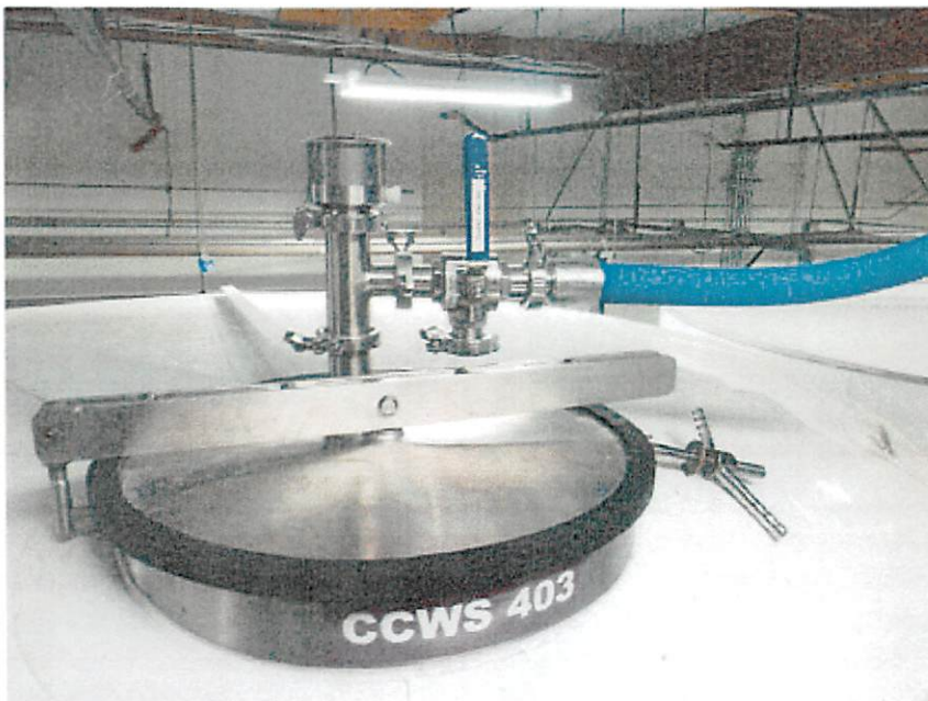
Closed top fermentation tank with EcoPAS piping
