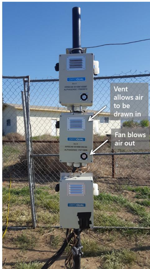
Figure 5. Housing for Alphasense and AirBeam sensors.
