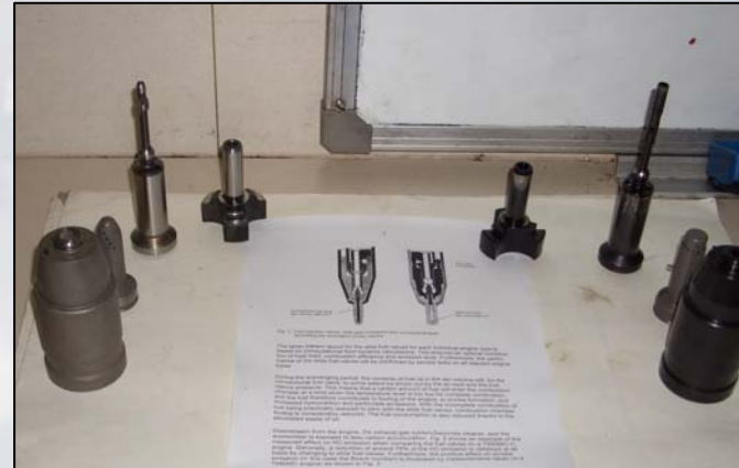
Cross sections of fuel-valve nozzle tips
